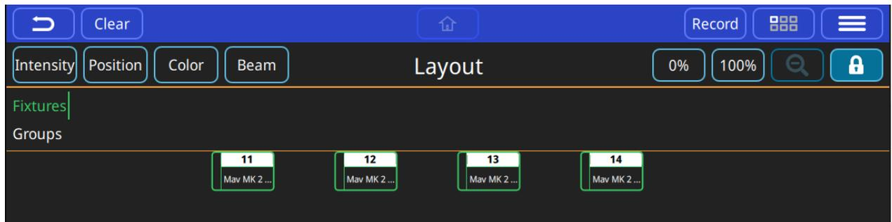
The larger fader on the left controls all currently selected instruments. You can also modify individual instruments by selecting them in this window.
