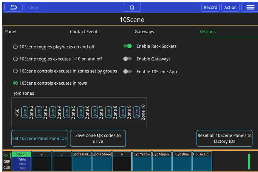
10Scene buttons can be used to toggle on and off **either** the first 10 execute buttons on the execute page, the 10 playbacks **or** using Zones to activate execute buttons in Zones.
