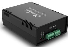
SnakeSys Gateway interfaces are used to connect 10Scene wall plates to a QuickQ Console or additional 10Scene wall plates to the QuickQ Rack. Each Gateway has 2 10Scene sockets to connect up to 20 10Scene wall plates (10 per socket) and 2 contacts.
